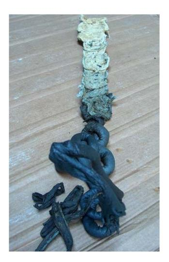
Especially developed for cleaning processing equipment of Amodel (PolyPhatalimide). Processing temperatures 315 - 350°C. Supernova HT-GF is a ready to use grade, with glass fibres.
